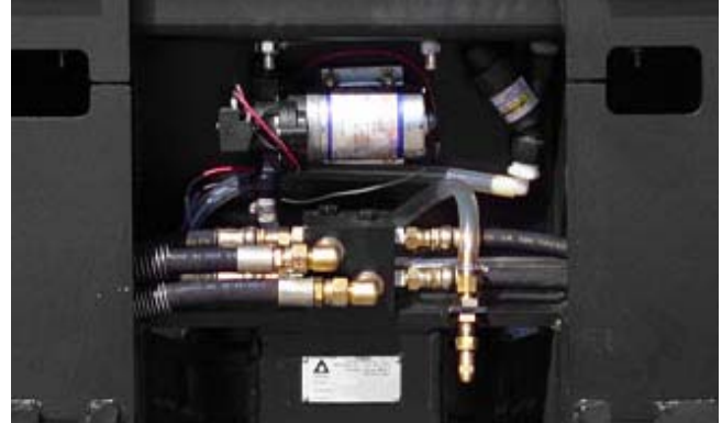
Dymax 14" Ranch Axe Tree Shear sprayer system eliminates re-growth of stubborn trees.
