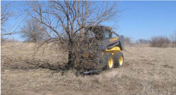
Photo Above: Dymax 14" Ranch Axe Tree Shear with hydraulic rotation. Supplied with diverter valve. Allows operators to rotate 90 degrees.
